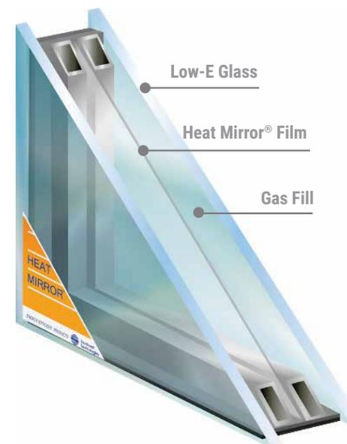
**Heat Mirror® Technology** suspends a lightweight polyethylene terephthalate (PET) film inside the airspace of a dual pane insulating glass unit to create multiple super-insulating cavities.
